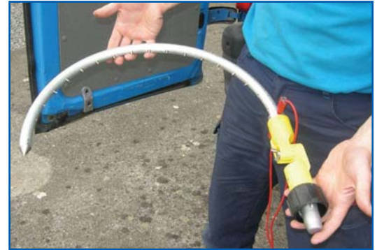
11. Arc clamp with connection cable (without telescopic crank)
