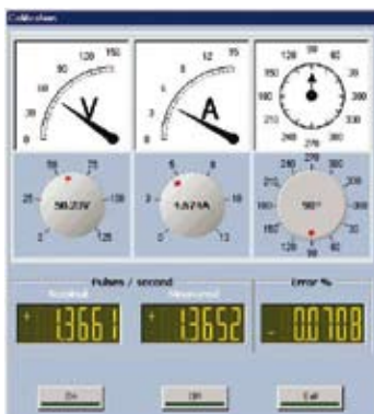
Energy Meter Test Program manual control.
