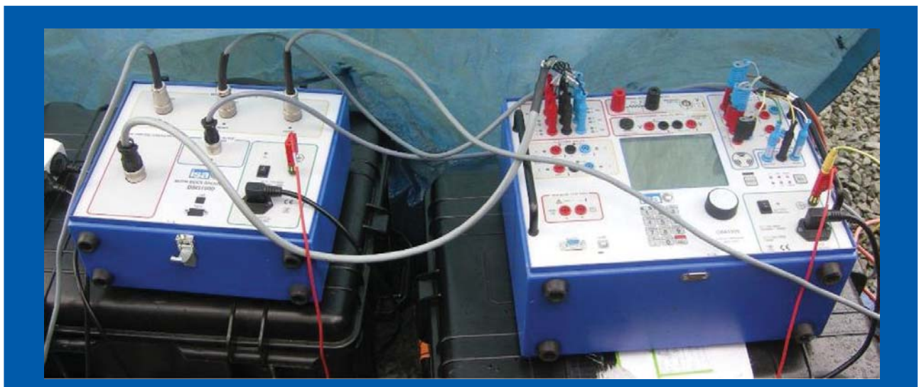
6. BSG 1000 connected to CBA 1000 during a test in a substation
