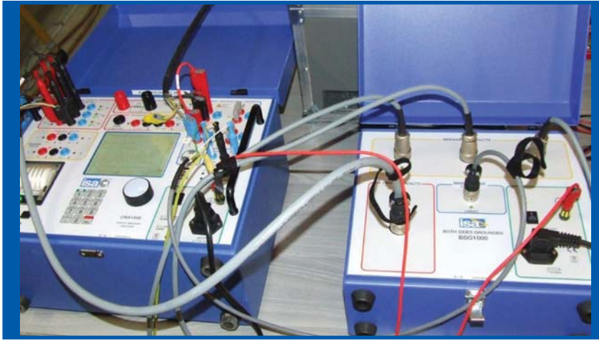
3. BSG 1000 connected to CBA 1000 during a real test
